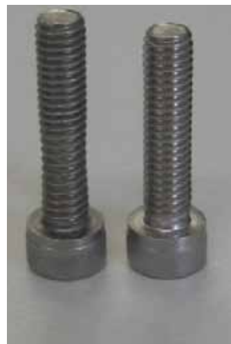
Left - bolt from Angie's mounting after 9 months use. Note the elongation of the bolt and the thinning around the neck of the bolt.
